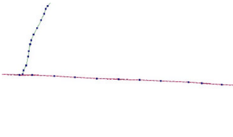
The second set of features was collected with a sub-meter system. No editing was needed. Notice the lack of any gap between the road segments and the consistency of the line.
