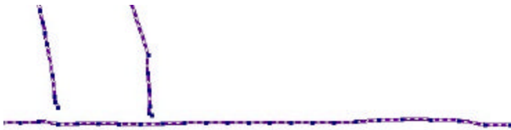
Figure 1. The first set of road features was collected with a 1-5 meter GPS system. With editing, the road features were acceptable. However, notice the gaps between segments and some of the inaccuracies (inconsistencies) showing up in the horizontal line.
