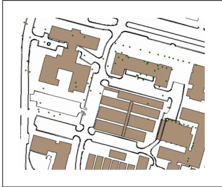
FIGURE 1: Tree data did not align with the survey accurate base map, notice tree point data appears on the shaded buildings and in roadways
